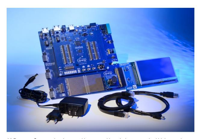
All Renesas Synergy development kits come with an industry standard high speed Segger J-Link OB debugger as well as an integrated Bluetooth<sup>®</sup> low energy (BLE) module.
